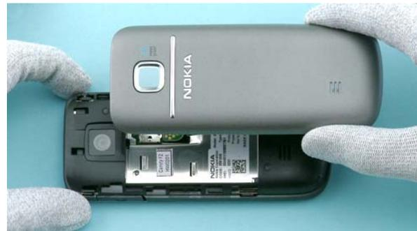
4) Remove the B-COVER ASSY. If there is a battery inserted, remove it also.
