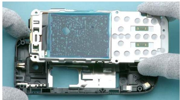
12) Remove the UI SHIELDING ASSY and the LIGHT SWAP PWB.
