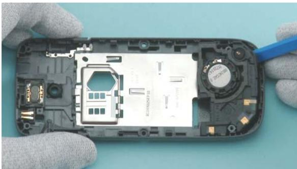
17) **Nokia 2730:** Use the SS-93 to lift up the ANTENNA MODULE from the D-COVER ASSY and then separate the module.
