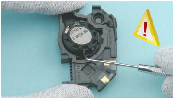
19) **Nokia 2730:** Detach the IHF SPEAKER with the dental tool and remove the speaker with the tweezers.
