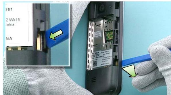
6) Place the SS-93 between the A-COVER ASSY and D-COVER ASSY. Detach the clips by sliding the SS-93 between the covers.
